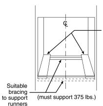
2 x 4 or equivalent runners level with bottom of cutout and flush with sides of cutout or solid bottom floor.
