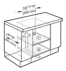
To route the water hoses and to ensure that the Combi Steam Oven has adequate ventilation, the following cut-outs measuring  $19 \, 11/16$ " x  $1 \, 9/16$ " ( $500 \, x \, 40 \, mm$ ) must be made:
