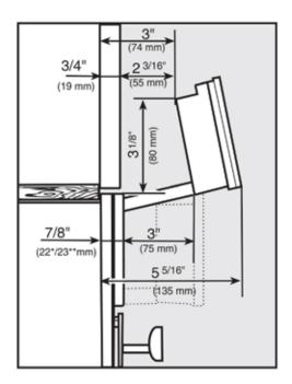
The area in front of the control panel must not be blocked by anything (such as a door handle) this would hinder the control panel from opening and closing.
