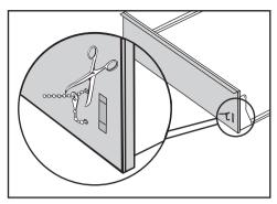
■ Remove the cable tie from the panel.
