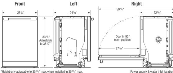
'Height only adjustable to 35 <sup>3</sup>/4" max. when installed in 35 <sup>3</sup>/4" max. standard cabinetry cutout. (Dimensions do NOT include insulation – insulation blanket may be compressed during installation.)
