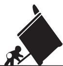
A child or adult can tip the range over and be killed. Verify that the anti-tip bracket is securely installed. Ensure the anti-tip bracket is engaged when the range is moved.
