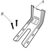
A. Anti-tip bracket B. #12 x 15%" screws (2)
