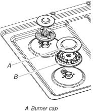
A. Burner ca<sub>l</sub> B. Burner
