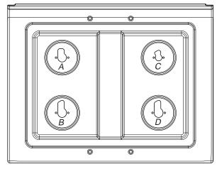
A. Standard burner - LP gas orifice spud number 88 (Yellow/Black) B. Power burner - LP gas orifice spud number 116 (Yellow/Orange) C. Simmer burner - LP gas orifice spud number 70 (Yellow/White) D. Power burner - LP gas orifice spud number 116 (Yellow/Orange)
