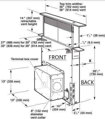
Note: Overall dimensions show unit with internal blower box attached. Remote Blower would only have a vent collar attached instead of the 13" x 13" box shown. X = Distance to the rear of the cabinet or wall. Must be a minimum of  $\frac{1}{2}$ ".
