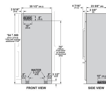
**NOTE:** GFI (ground fault interrupter) is not recommended. Water line can enter the opening through the floor or rear wall. The water line installed should be 1/4" O.D. copper tubing or GE SmartConnect<sup>™</sup> tubing between the cold water line and water connection location. The line should be long enough to extend to the front of the refrigerator. Installation of an easily accessible shutoff valve in the water line is required.
