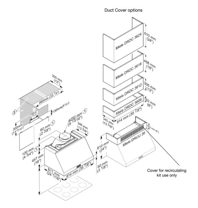
The hood with exhaust collar is only used in vented mode with an internal or external blower.
