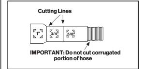
• If a longer drain hose is required, add up to 42" of length for a total of 10 ft. to the factory installed hose. Use 5/8" or 7/8" inside diameter hose and a coupler to connect the two hose ends. Secure the connection with hose clamps.
