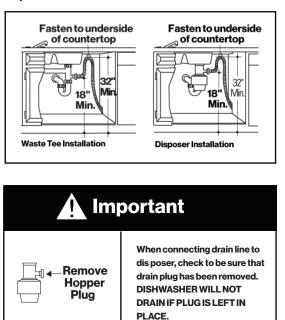
**TIP:** Avoid unnecessary service call charges. Always be sure disposer drain plug has been removed before attaching dishwasher drain hose to the disposer.
