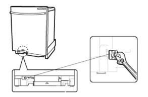
• Do not over tighten 90° elbow water valve bracket could bend or water valve fitting could break.
