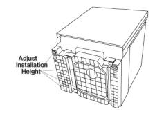
• Measure installation height and dishwasher height. Extend leveling legs out from the dishwasher base, 1/4" less installation height.
