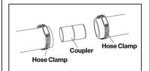
• Secure the drain hose to the air gap, waste tee or disposer with clamps.
