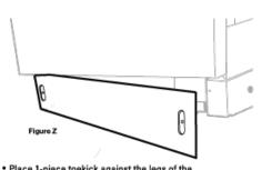
Place 1-piece toekick against the legs of the dishwasher. The slots should align with toekick bracket screw holes. Allow the toekick to touch the floor. Install the toekick screws.
