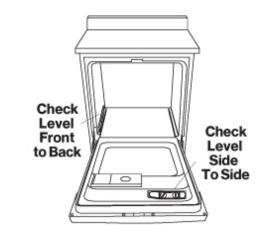
• Level the dishwasher by adjusting the four leveling legs individually.
