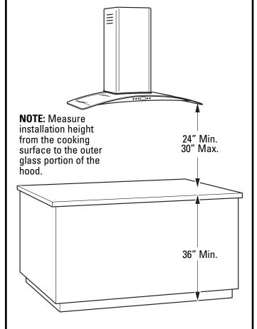
The vent hood must be installed 24" min. and 30" max. above the cooking surface. The hood installation height, from the cooking surface to the bottom of the hood, depends upon ceiling height.
