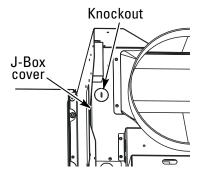
Secure the house wiring to the junction box with a strain relief.
