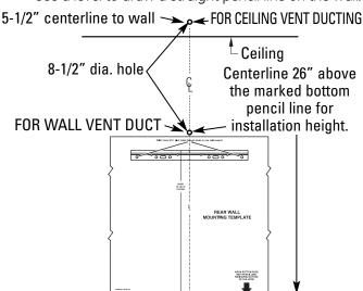
Tape the template in position along the penciled line. CHECK TO BE SURE THE TEMPLATE IS LEVEL.
