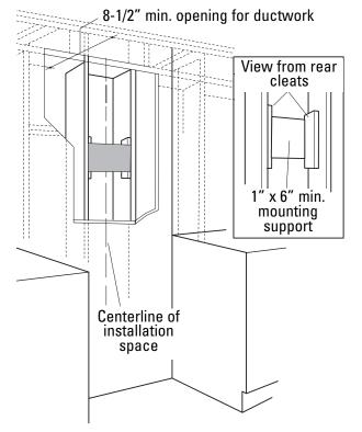
If drywall is present, mark the screw hole locations for the top mounting brackets. Remove the template.
