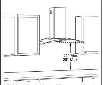
NOTE: Installation height should be measured from the cooking surface to the outer glass sides.
