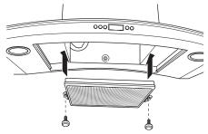
• Install the black charcoal filter into the center opening. Secure the filter with thumbscrews on each side.
