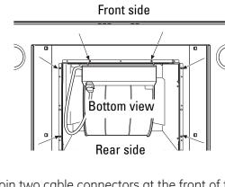
• Join two cable connectors at the front of the hood.
