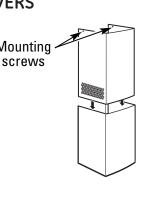
The inside duct piece must slip into the folded ends of the outer section.
