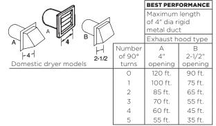
For every extra 90° elbow, reduce the allowable vent system length by 10 ft.
