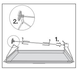
Insert the pointed end of the rotisserie (1.) into the motor slot at the back of the rotisserie set up and set the other end onto the holder (2.) as illustrated.
