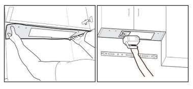
Caution: Wear safety goggles when drilling. In case of batten at the wall facing the bottom plate, the rear wall side of the paper template shall be cut as per the thickness of the batten.
