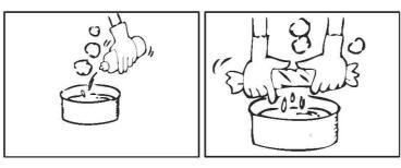
Washing and cleaning the surface, Grease Cup, and grease filter: (The cleaning can be done by the user)
