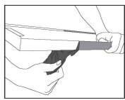
7. Lift and position the hood onto the brackets at the bottom of the backside while keeping an angle between the wall and the hood, and then push the hood against the wall tightly.
