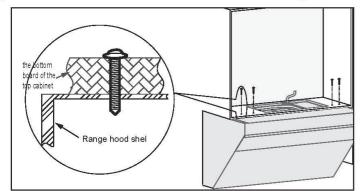
If there is a big gap between the bottom board of the top cabinet and the top of the range hood, please add wood pads based on the gap size near the four M5×70 screws to avoid range hood shell deformation caused by the tightening of screws, which will affect the use of the range hood.
