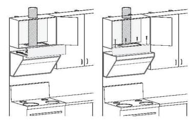
10. Make sure the hood is leveled. Install the Grease Cup, and plug the appliance for a test run.
