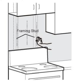
3. Locate the duct bracket. Determine the central point and mark the centerline on the wall where the hood will be installed. Also, mark the point where the central line and the lowest point on the bottom board of the top cabinet meet. This is the location, in which to secure the bracket. Mark screw hole locations on the wall. The distance between the lowest point on bottom board of the top cabinet and the center of the bracket should be 16" (405mm).
