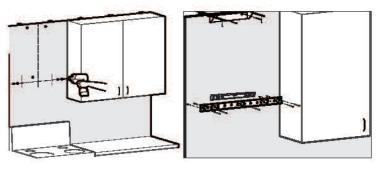
Caution: One of the screws for duct bracket must be fastened to the wooden beam.
