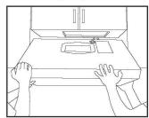
8. Secure the hood to the upper cabinet with four M5 X 70 fastened screws for upper cabinet. The hood will need to be supported before you loose your hands until at least two screws are tightened.
