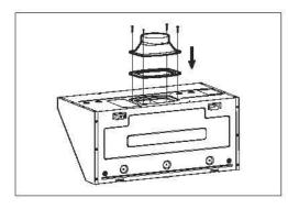
8. Lift and position the hood onto the brackets at the top of the backside while keeping an angle between the wall and the hood, and then push the hood against the wall tightly. Secure the duct to the duct cover and seal the connection with aluminum tape.
