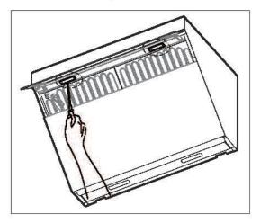
4. Disconnect the wires and then replace the LED lights.
