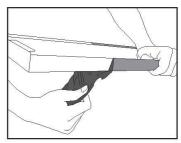
7. Place the gasket seal on the hood outlet and fix the duct cover with four M4 x 18 screws of outlet housing.
