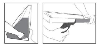
7. Lift and position the hood onto the mounting screws. Make sure the hood is stable and leveled by using a spirit level. Install the safety buffer baffle above the hood.
