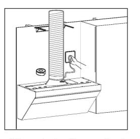
9. Tear off the protective film over the decorative cover and the blower housing; then install the decorative cover onto the brackets. Push the blower housing downward and lock it to the cover screws.
