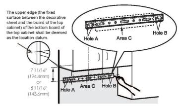
4.Fasten the bracket: drill Ø8 hole at the screw hole marks with electric drill, embed expansion tubes and fasten the bracket with bracket screws. Use leveling instrument to make sure that the bracket is leveled.
