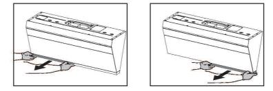
Warning: For the safety of you and your family, please regularly clean the oil accumulated in the Grease Cup and deposits on the Grease Cup surface. Do wear qualified protective gloves.
