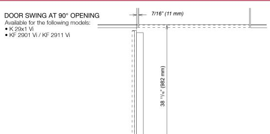
NOTE: Additional space needed depending on thickness of front panels and handle used
