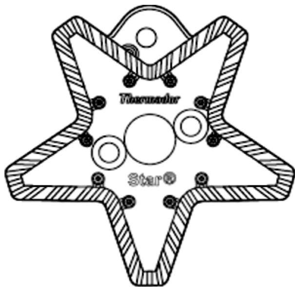
Figure 8: Star® Brass Burner Base
