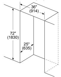
Leave 1/2" (12.7) gap at the top and 1" (25.4) behind the refrigerator for proper ventilation.
