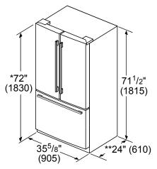
\*Add <sup>5</sup>/8" (17) with front leveling feet fully extended \*\*Add 1" (25) for fixed spacers on back
