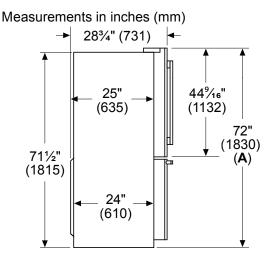
A: Add <sup>5</sup>/8" (17) with front leveling feet fully extended
