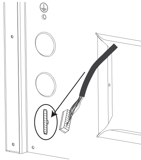
Figure 17: Pigtail Remote Connection
