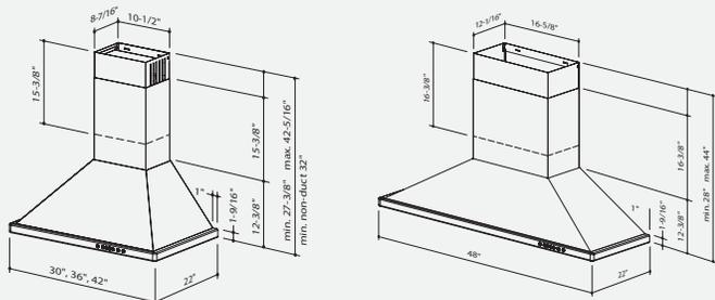
Reversible telescopic flue allows non-ducted recirculation.
