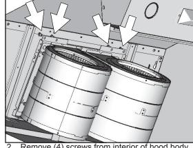
Remove (4) screws from interior of hood body attaching blower plate to top of hood body.
