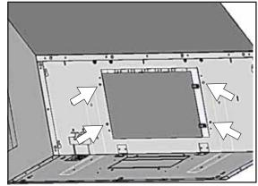
From inside hood body, position top cover plate to top of hood body. From outside hood body, attach top cover plate to top of hood body using (4) 3/16 x 3/8 screws.
