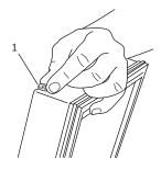
Using a Phillips screwdriver, remove the two screws holding the custom stainless handle from the original location, and remove the handle. Remove the two screws on the opposite side of the door. Do not place handle on door until you have completed, steps 9 & 10.
