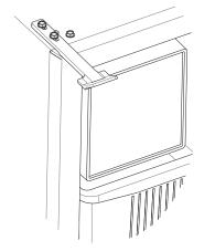
14.Place the door latch assembly on opposite side of unit. Be sure to tighten all three screws securely.
