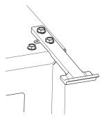
15. Place door on lower hinge pin. Invert and install upper hinge on door. Fasten upper hinge to unit (three screws). Partially tighten screws.
