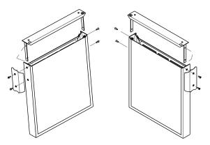
Remove plastic hole plug from door handle and relocate on opposite side. Lift the handle slightly and press on the locking tab, then gently pry the hole plug out of the hole being careful not scratch the top cap.
