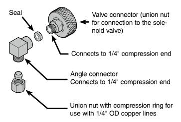
The connection to the valve connector can be done with or without the angle connector, as required.
