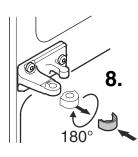
8. Remove hinge bushing, turn through 180° and re-fit.
