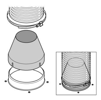
If you would like to reduce the environmental impact of your ventilation system by limiting the CFM output the Reducing Collar can be installed. It reduces the air flow to less than 400 CFM. Check local building codes for maximum CFM requirements.
