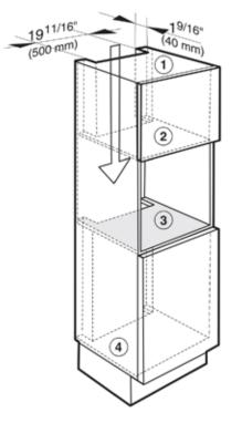
To route the water hoses and to ensure that the Combi Steam Oven has adequate ventilation, the following cut-outs measuring  $19 \ 11/16" \times 1 \ 9/16"$  (500 x 40 mm) must be made:
