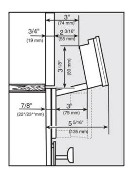
The area in front of the control panel must not be blocked by anything (such as a door handle) this would hinder the control panel from opening and closing.
