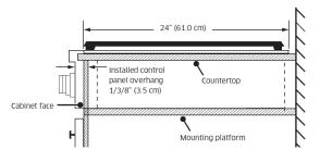
Installed Rangetop - Side View
