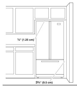
To ensure proper ventilation for your refrigerator, allow for a 1/2" (1.25 cm) of space on each side and at the top. Allow for a 1" (2.54 cm) space behind the refrigerator. If your refrigerator has an ice maker, allow extra space at the back for the water line connections. When installing your refrigerator next to a fixed wall, leave a  $3^{3}/_{4}$ " (9.5 cm) minimum space between the refrigerator and wall to allow the door to swing open.
