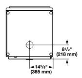
**NOTE:** Most installations require a minimum of 6" (152 mm) clearance behind dryer for exhaust vent with elbow. See "Venting Requirements."
