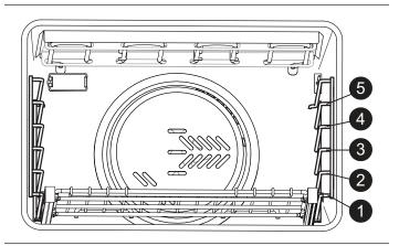
Figure 27: Oven Rack Positions
