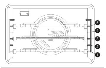
Figure 1: Main Oven Rack Positions
