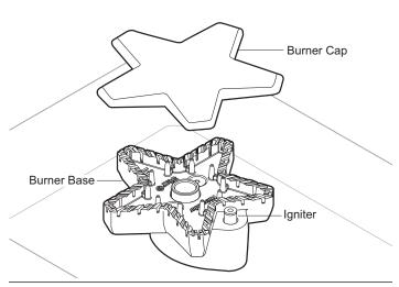
**Figure 13: STAR Burner Components**
