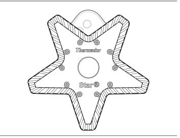
Figure 9: STAR Brass Burner Base
