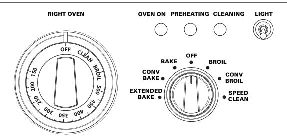
Figure 29: Oven Controls for 48" Range Main Oven
