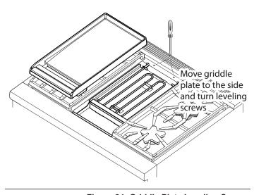
Figure 24: Griddle Plate Leveling Screws
