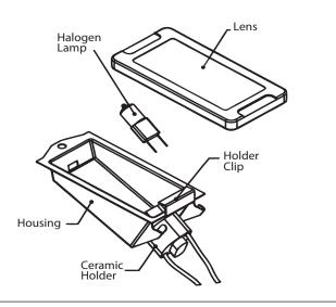
Figure 31: Oven Lamp Assembly
