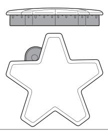
**Figure 14: Correct Burner Cap Placement**
