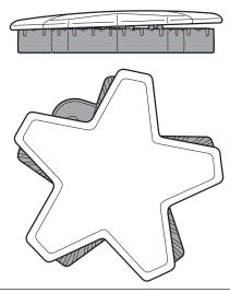
Figure 15: Incorrect Burner Cap Placement
