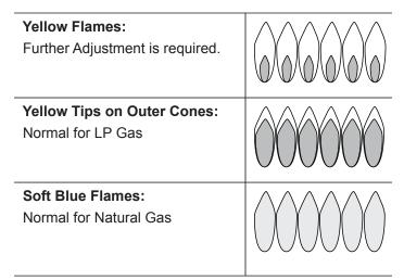
If the flame is completely or mostly yellow, verify that the regulator is set for the correct fuel. After adjustment, retest.
