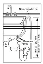
Note: Plumbing installations will vary - refer to local codes. Drain hose included is  $90\,1/2$ " (230 cm) and can be extended to a maximum of  $168\,1/2$ " (428 cm).
