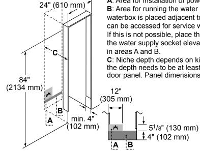
A: Area for installation of power connection.
