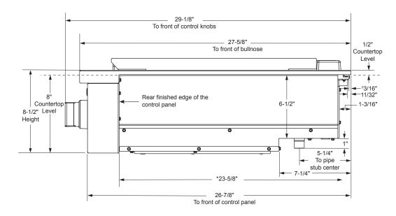
\* Minimum cabinet cutout depth from the back of the rear trim to the back finished edge of the control panel typically, the minimum cabinet depth (front to back). Maximum cabinet cutout depth is 26" minus the countertop overhang. † Include the overhang of the rear trim when countertop continues behind the product.
