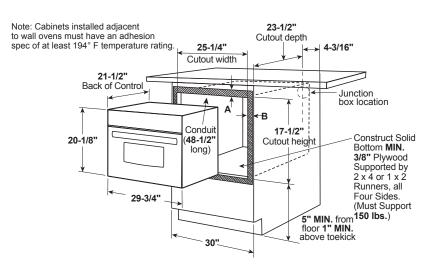
A= Allow 1" overlap of oven over bottom edge of cutout, and allow 2-3/4" overlap at top edge of cutout.
