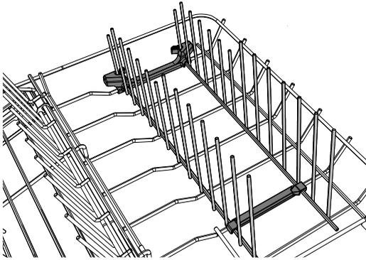
Release by pushing the small clips at the rear and fold the tine sections down towards each other.
