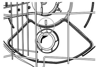
Line up the arrows on the filter plate and insert the drain filter
