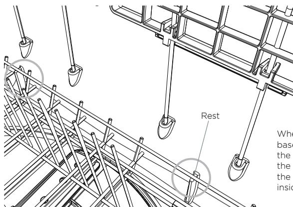
When refitting the base rack, ensure the outer edges of the rack sit on all the rests within the inside of the drawer.
