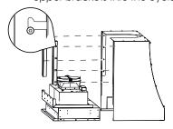
3 Secure the insert hood to the lower support.
