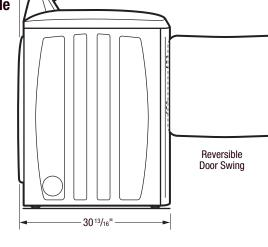
back. To achieve 6" minimum rear clearance, dryer installation requires 2" minimum clearance between front of unit and vented door. Door MUST be vented with 120 sq. in. minimum louvered opening, equally full-length of door is acceptable. Air openings MUST remain unobstructed with door installed. For additional installation details, refer to Product Installation Guide on web.
