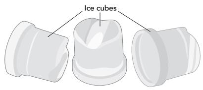
Normal cubes are tapered cylinders. If the cubes are ragged and misshaped, mineral scale must be removed from the ice making system.
