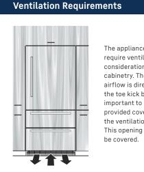
The appliance do not require ventilation considerations in the cabinetry. The required airflow is directed through the toe kick base. It is important to use the provided cover grille for the ventilation opening. This opening must not
