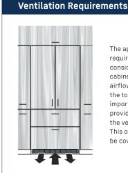
The appliance do not require ventilation considerations in the cabinetry. The required airflow is directed through the toe kick base. It is important to use the provided cover grille for the ventilation opening. This opening must not be covered.
