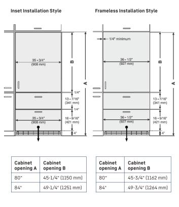
Minimum panel thickness is 5/8" (16 mm).
