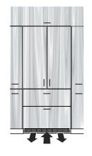
The appliance do not require ventilation considerations in the cabinetry. The required airflow is directed through the toe kick base. It is important to use the provided cover grille for the ventilation opening. This opening must not be covered.
