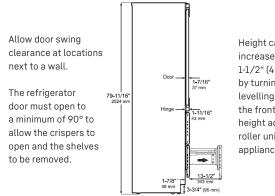
Height can be increased by 1-1/2" (40 mm) by turning the levelling feet at the front and the height adjustable roller units at the appliance rear.
