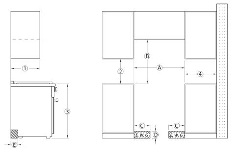
(c), (c), (c) The shaded area represents the installation area for the connections: (c) E = Electrical connection, (c) W = Water connection, (c) G = Gas connection
