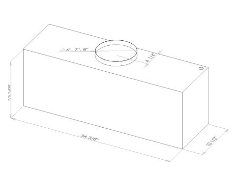
Note: Electrical access located on the top, right side as shown in the above dimensioned diagrams.
