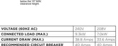
**NOTE:** Check local codes for required breaker size.
