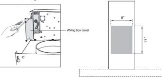
If the power cord to connect the hood to the main power comes from the wall in the grey area (8"x17"), it must have a minimum lenght of 20" to be connected to the Junction Box.
