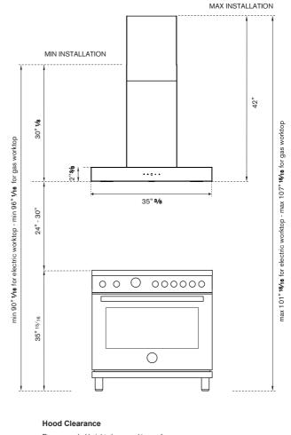
Recommended height above cooking surface: min 24" for electric worktop min 30" for gas worktop
