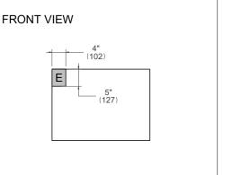
For single ovens installed into a wall cabinet, the electrical junction box may be located above, below to the left or right of the unit within reach of the power cord.
