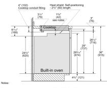
Dimensions based on standard countertop height (36" with  $4^{3}\!/\!4"$  toe kick including base plate).
