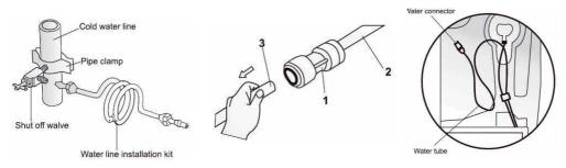
**CONNECT WATER VALVE:** Connect water supply line to water valve with accessible shutoff valve. Connect water line to refrigerator using installation kit. Kit includes one water tube and connector. Second water tube not supplied. Connect first water tube [2] into corresponding hole of water connector[1].
