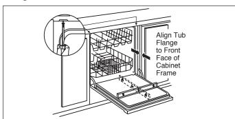
Fasten the dishwasher to the underside of the countertop with the 2 Phillips screws provided.
