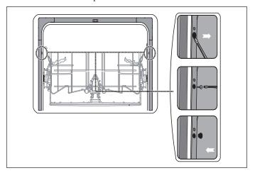
**IMPORTANT** Drive screws straight and flush. Protruding screw heads will scratch the top of the control panel and can interfere with the door's ability to close. If the gap is less than 3/8" between control panel and the screws, method 2 is recommended.
