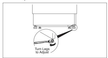
**TIP:** Pull lower rack out, about halfway. Make sure the rack does not roll forward or back into dishwasher. If the rack rolls in either direction, the dishwasher must be leveled again.
