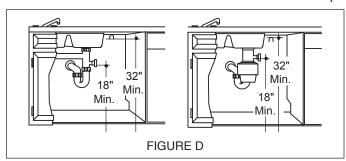
Install waste tee or disposer and air gap according to manufacturer's instructions.
