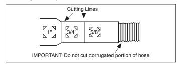
• If a longer drain hose is required, add up to 42" of length for a total of 10 feet to the factory installed hose. Use 5/8" or 7/8" inside diameter hose and a coupler to connect the two hose ends. Secure the connection with hose clamps.
