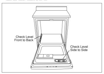
• Level the dishwasher by adjusting the four leveling legs individually.
