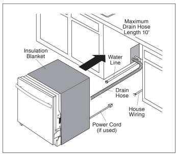
**TIP:** Position water line and house wiring on the floor to avoid interference with base of dishwasher.
