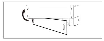
• Place 1-piece toe kick against the legs of the dishwasher. The slots should align with toe kick bracket screw holes. Allow the toe kick to touch the floor. Install the toe kick screws.
