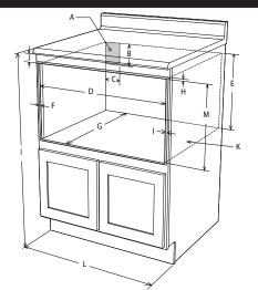
24" CONVECTION MICROWAVE DRAWER FLUSH MOUNT MEASUREMENTS
